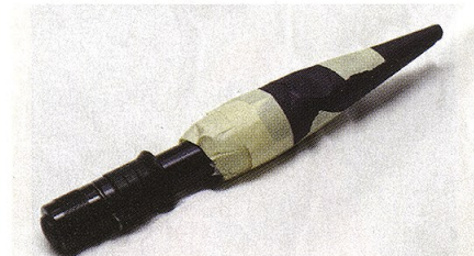
Black construction paper is used to make a narrow aperture light source.
